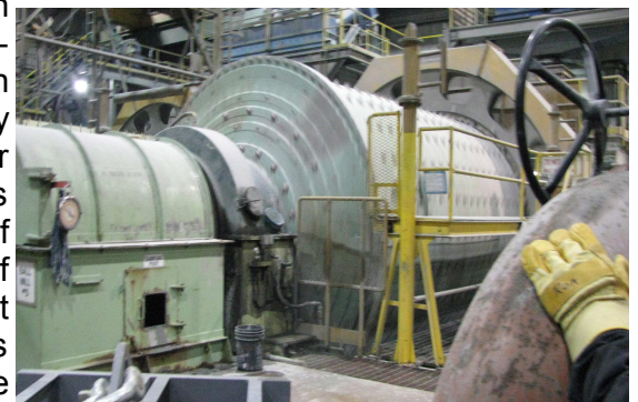
the 'ball drums' used to breakdown the rocks
